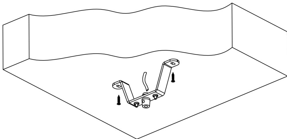
**EN** 1. Mount the lamp bracket on the ceiling \*.
